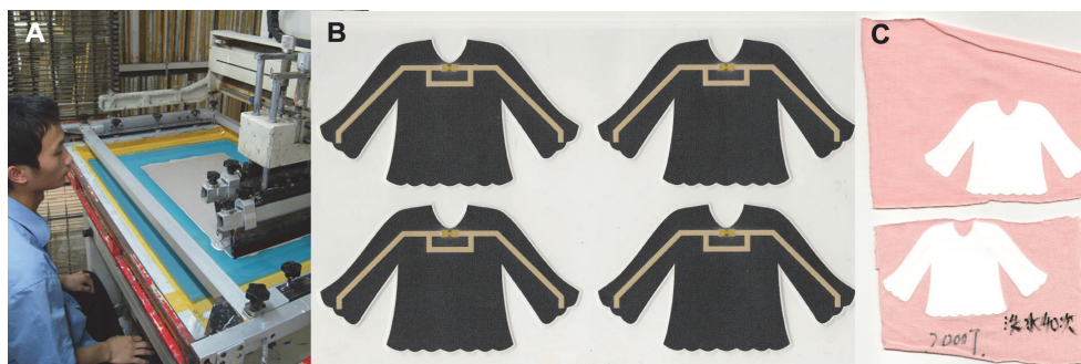
Fig. 2. Photographic images showing the RFID tag incorporated high reliability hot-press labels for garments. A) A worker is screen-printing the ultralow cost ECA based antenna in his work line in a company in Dongguan, China; B) A group of labels ready for heat-transfer printing; C) Samples cotton fabric pieces with the labels heat-transferred onto them. (Upper: before washes; bottom: after washing for forty cycles.) The RFID read range performance remained the same after the heat-transfer process and the subsequent washing cycles.
