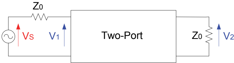
Fig. 8. Circuit topology used to measure S-Parameters.
