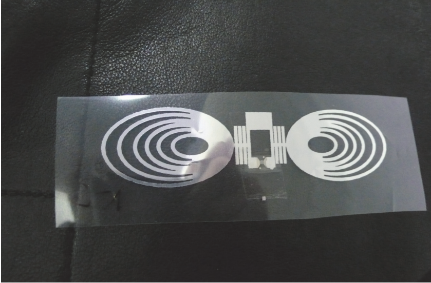
Fig. 14. A tag antenna using a company logo
