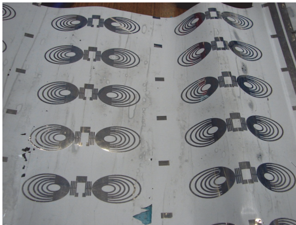
Fig. 7. A hybrid method with gravure printing and vacuum deposition technology
